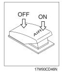
(1) This switch is used to activate the air compressor.
